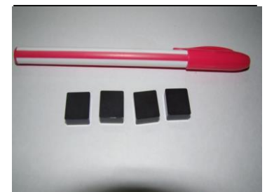
Cutting tool inserts of configuration SNGN120408
